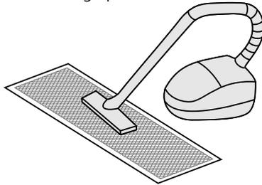
Clean the filter with clean water (except for the activated carbon module), with the air inlet side of the filter facing downwards.
