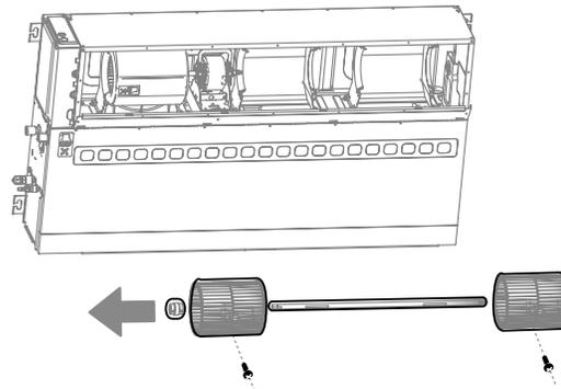
**07.03.07. Maintenance of the bearing block (model with 3 fans)**
