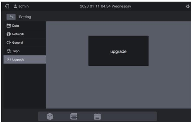
Click "Upgrade" and select the package to be upgraded in the pop-up interface. The centralized controller will automatically restart and upgrade the firmware.
