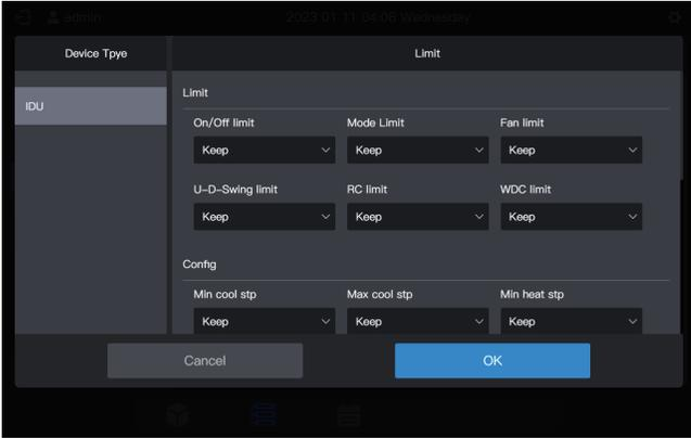
Note: When an extension command is sent, it takes a certain amount of time for the centralized controller to refresh the latest state of IDUs. The specific amount of time depends on the number of connected devices. (According to laboratory test data, when the connected devices are 8 refrigerant systems and 64 IDUs, the maximum polling cycle lasts for about 15 minutes. The actual duration may vary.)
