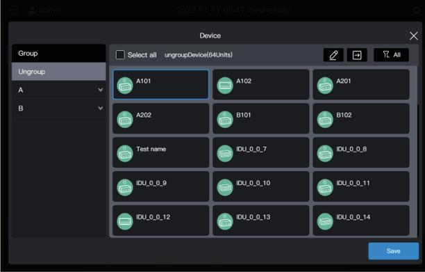
Note: Immediately after the centralized controller is debugged, all IDUs are in "Ungroup".
