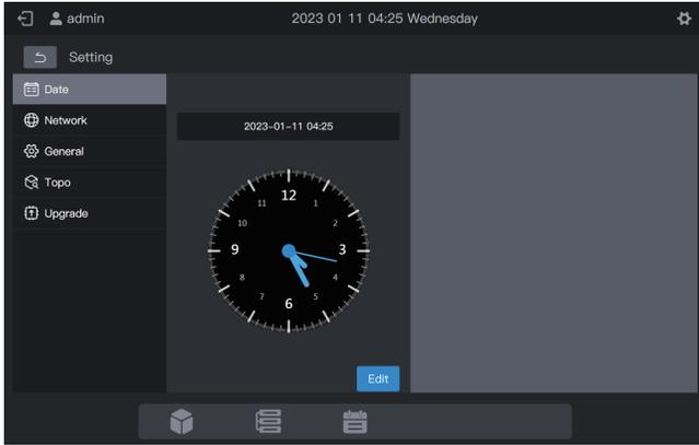
In the "Date Setting" module, you can set the date of the centralized controller. Click "Edit". Then, the centralized controller enters the date setting state. At this time, the clock will stop and not start until the controller exits the date setting state.
