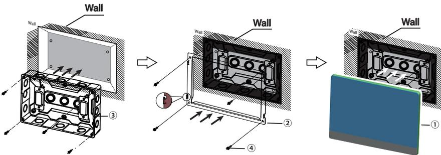
Attention: The controller is only suitable for installation at a height of  $\leq 2m$ .
