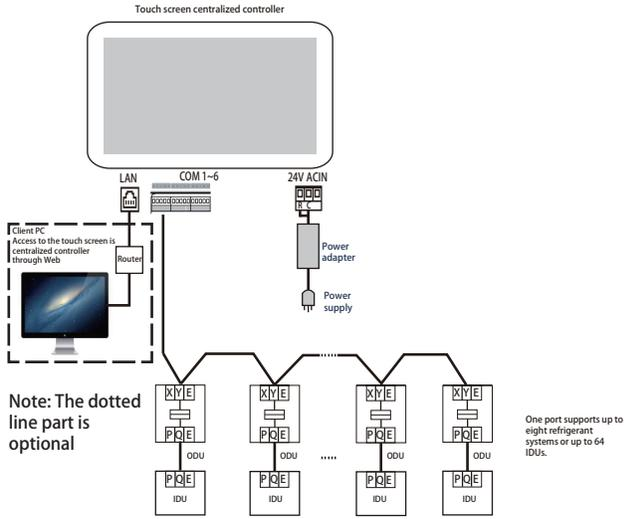
Note: There may not be a PQE interface between an IDU and an ODU. For details, refer to the manual of ODU and IDU. This is only used to illustrate the centralized controller framework.
