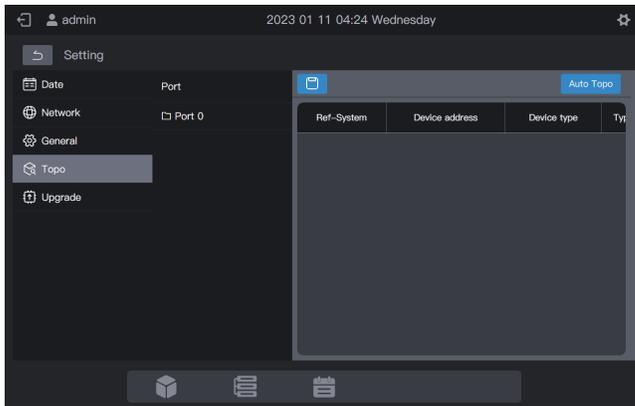
To use the centralized controller for the first time, you need to search for the device connected to it before the controller displays that device.
