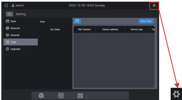
Click "Topo" in the left menu and "Auto Topo" in the right area. The centralized controller will start to obtain information about the refrigerant system connected to the centralized controller and automatically construct the topological relationship. After this, the interface will appear as follows:
