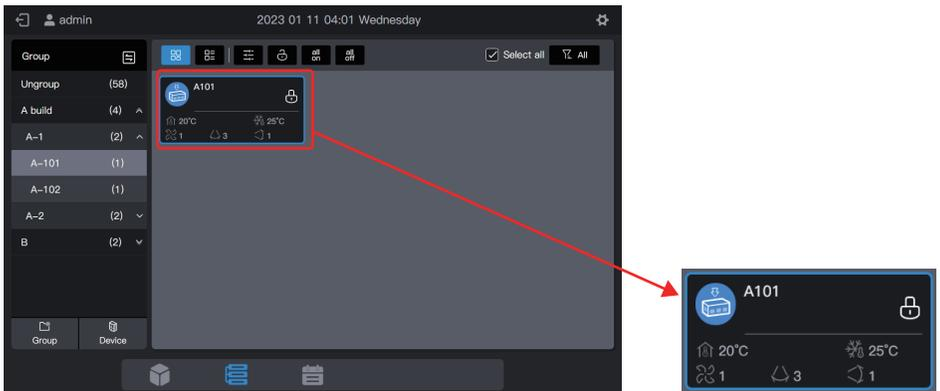
In the list display state, select the IDU by checking the selection box in the first column of the list box.
