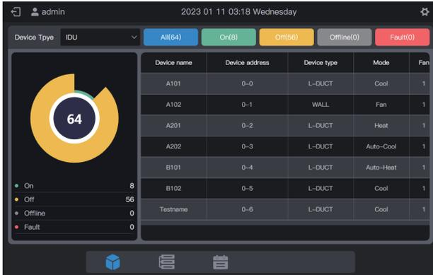
View the status distribution and general parameters of IDUs. When there are multiple types of access devices, you can view the status of different types of devices through "Device Type".
