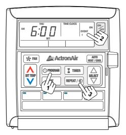
This feature allows you to automatically repeat the previous days, events and times, therefore eliminating the need to re-enter the events and times.
