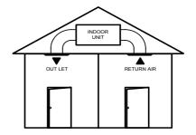
Dust off the outlets and return air, use a household duster. Do this regularly to prevent any build up of dust or dirt.
